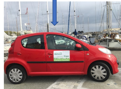
Peugeot 107 City Car runs on 105 Octane M85 methanol made from Danish biogas. Info sheet.
