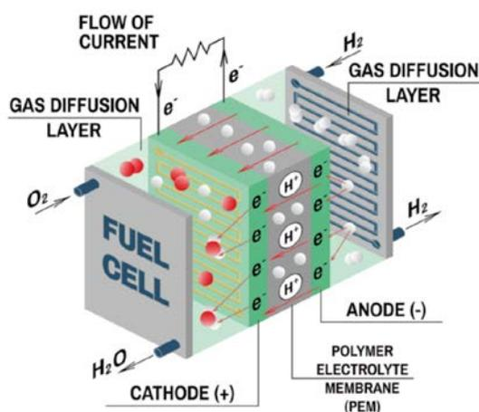
The HT PEM-technology is characterized by simple heat management and a minimum balance of plant components which in turn reduces the parasitic losses to run the system. The simple system design enables a high total system power density although the stack power density is lower than generic stack designs.
